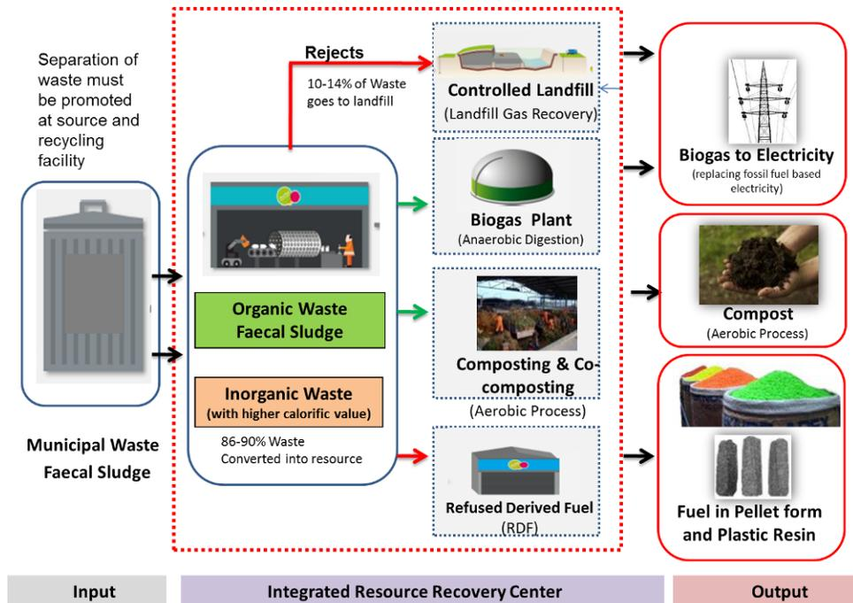
Figure 2: Shows the Concept of Integrated Landfill and Resource Recovery Center (IL&RRC)
