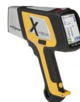
We use our XRF analysing device (X-Ray Fluorescence). Mainly the metals can be found with this method. If the screening shows something we go on with external laboratories to verify our findings.
